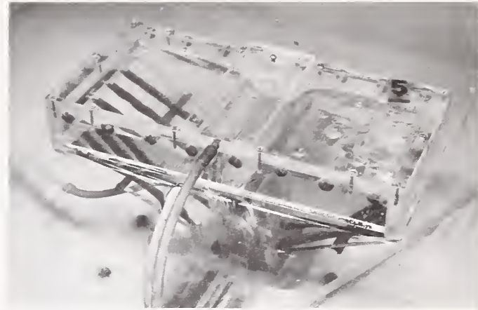
FIGURE 12.—Vents closed, head -0.8 ft, discharge 229 c.f.s. Siphon-regulated flow, air entering from under antivortex plate skirt, drop inlet partly full.
